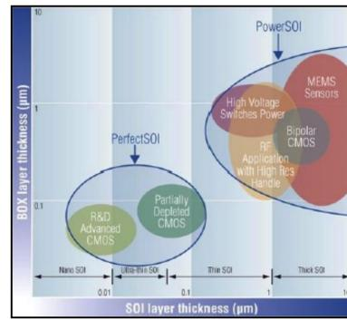
Fig. 2: An example of SOI types and applications from SunEdison Semi, a major manufacturer of SOI wafers, PerfectSOI = thin and PowerSOI = thick.
