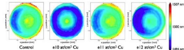
Fig. 8: SR Top Si Film Thickness Maps for 1500/1000 nm SOI.
