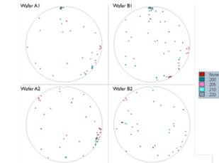
Figure 11: Surfscan surface defect results on 12/25 nm SOI.
