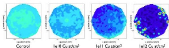
Fig. 10: SHG maps of 1500/1000 nm SOI wafers after parsing layer thickness.
